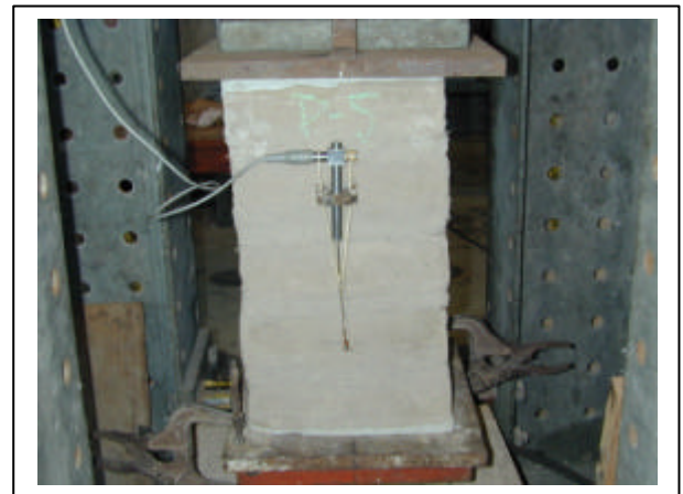
Figure 15b. Axial compression test.
