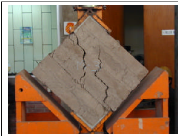
Figure 15a. Diagonal compression test.
