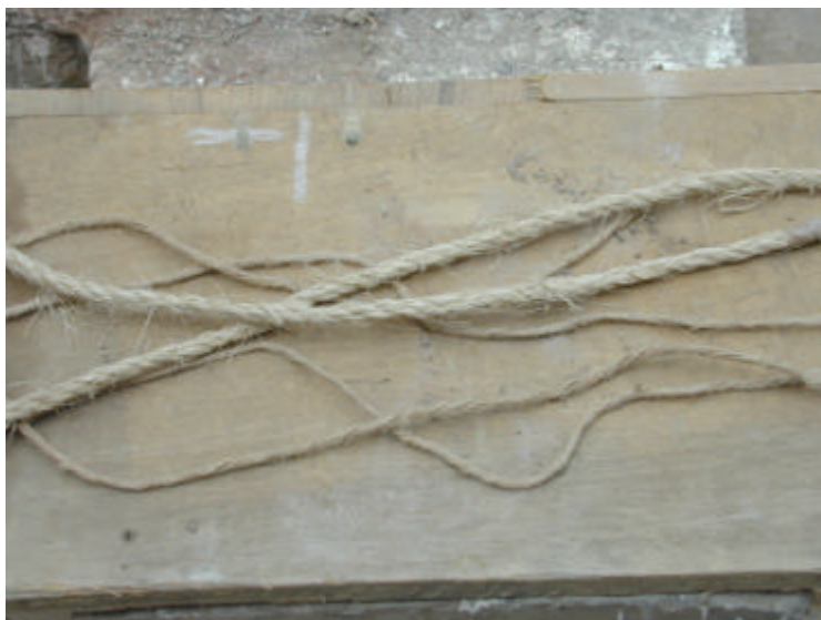
Figure 4. Cabuya rope for horizontal reinforcement and yute thread.
