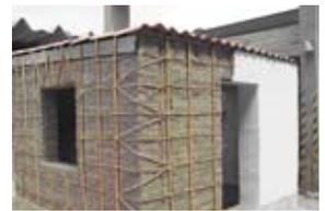
Cane reinforced adobe structure before test
